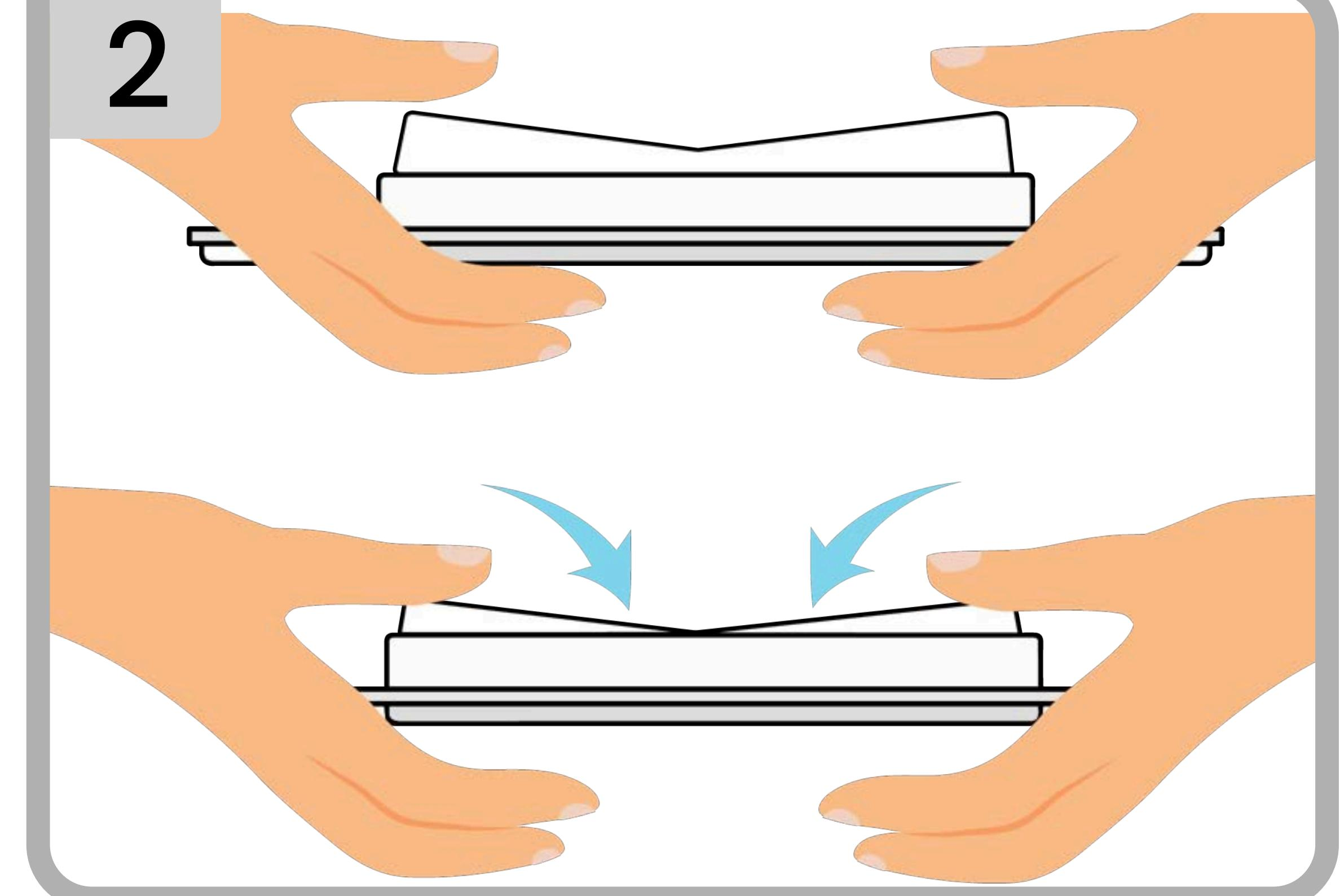
**EN** Squeeze and release both ends of the switch simultaneously.
