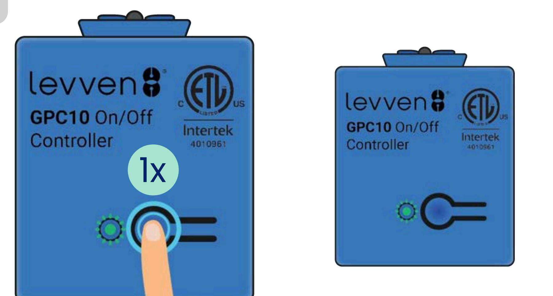
**EN** Press and release the pair button on the first controller again to complete grouping. Its LED will flash green 3 times to confirm the grouping.
