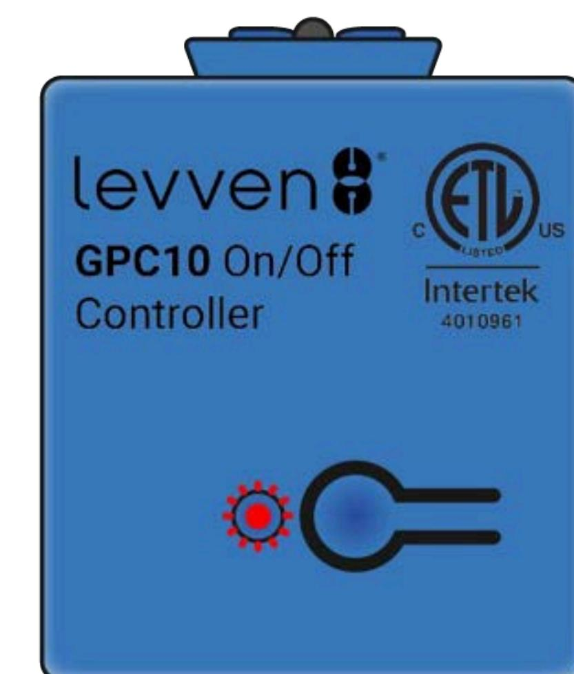
**EN** To clear the controller's switch pairings, press and hold the pair button for 5 seconds.
