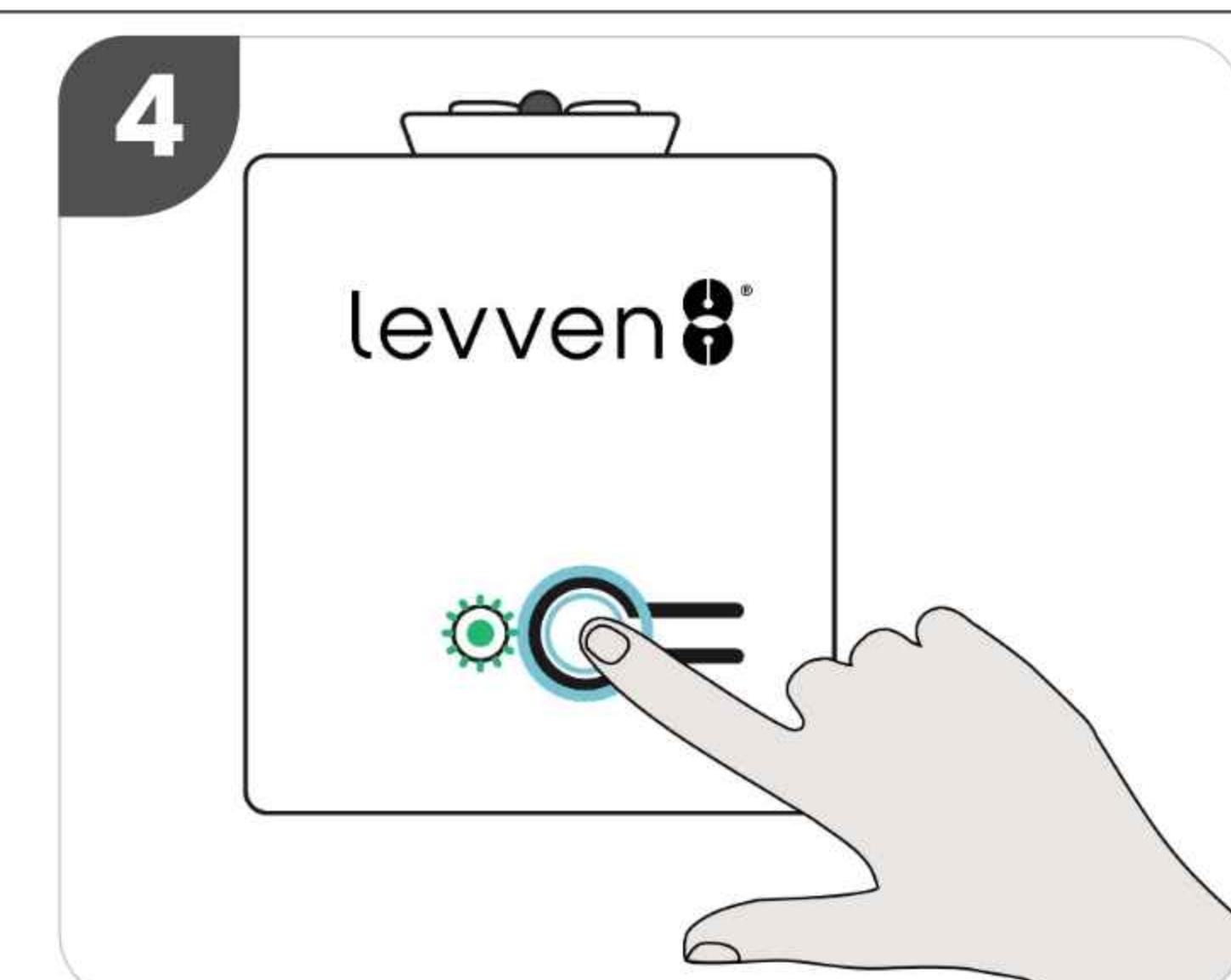
Press and release the pair button on the controller to complete pairing. The LED flashes green 3 times if pairing is successful; otherwise, it flashes red. If the pairing was unsuccessful, restart from Step 1.
