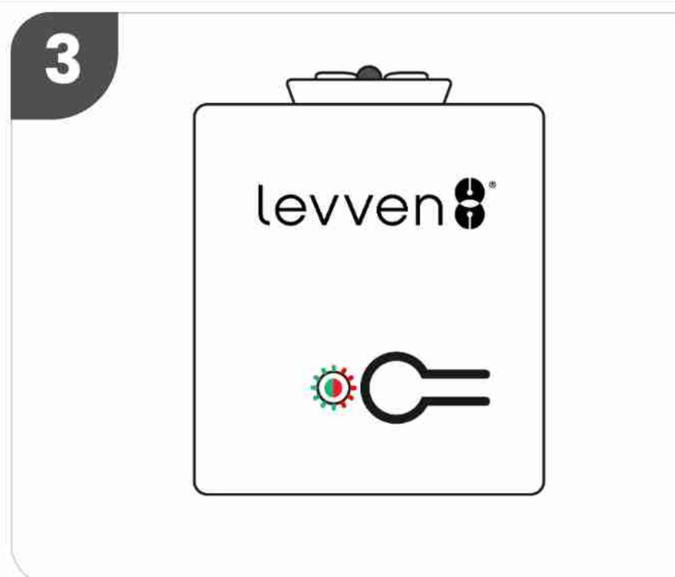
The LED on the controller will start blinking red and green to confirm a signal is received.
