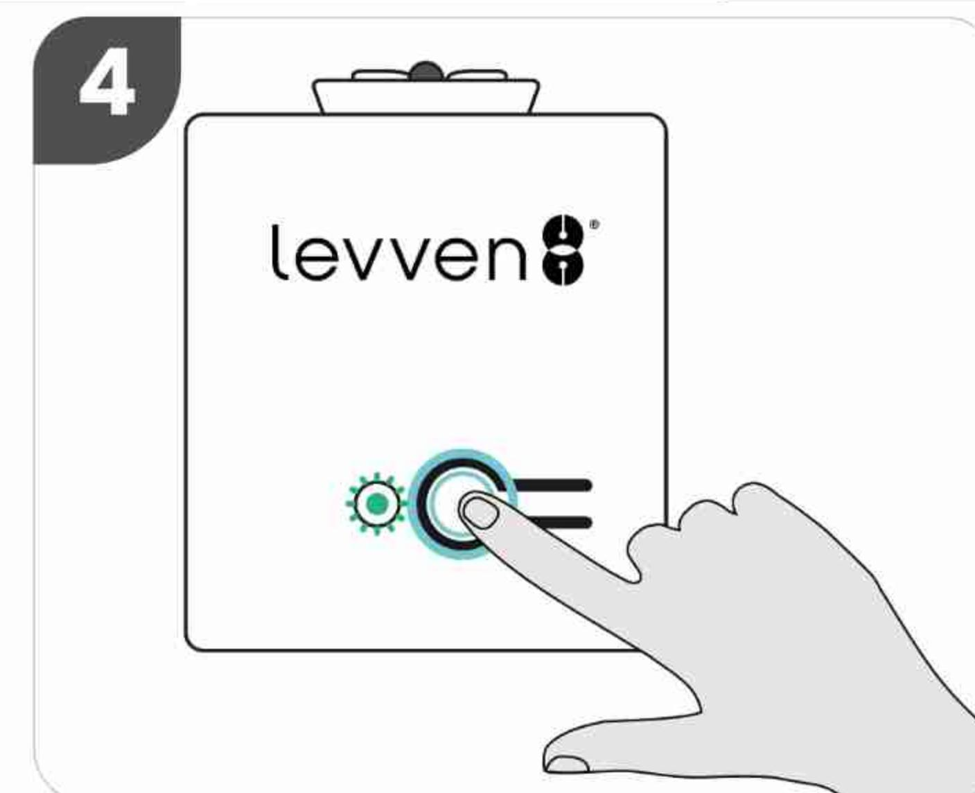
Press and release the pair button on the controller to complete pairing. The LED flashes green 3 times if pairing is successful; otherwise, it flashes red. If the pairing was unsuccessful, restart from Step 1.
