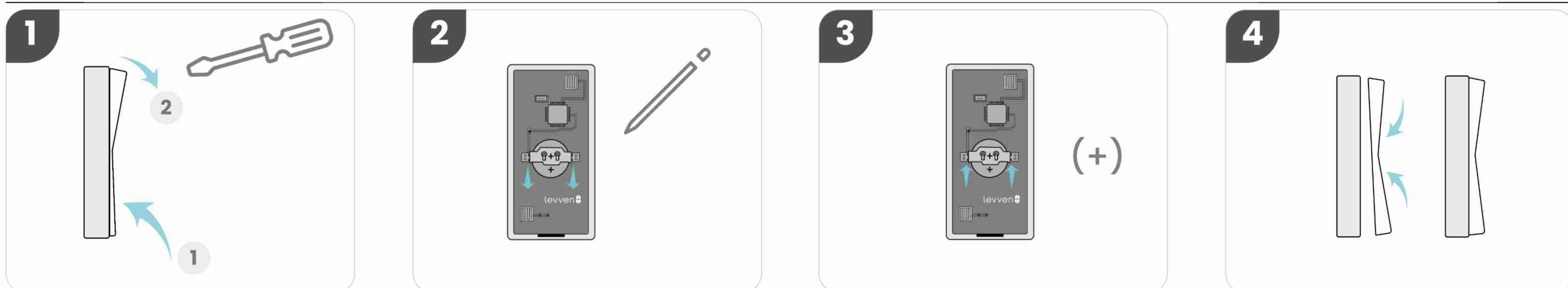
**Press and hold the bottom or top of the switch rocker. Use a screwdriver or similar tool to pry the switch rocker off the switch to reveal the battery compartment.**
