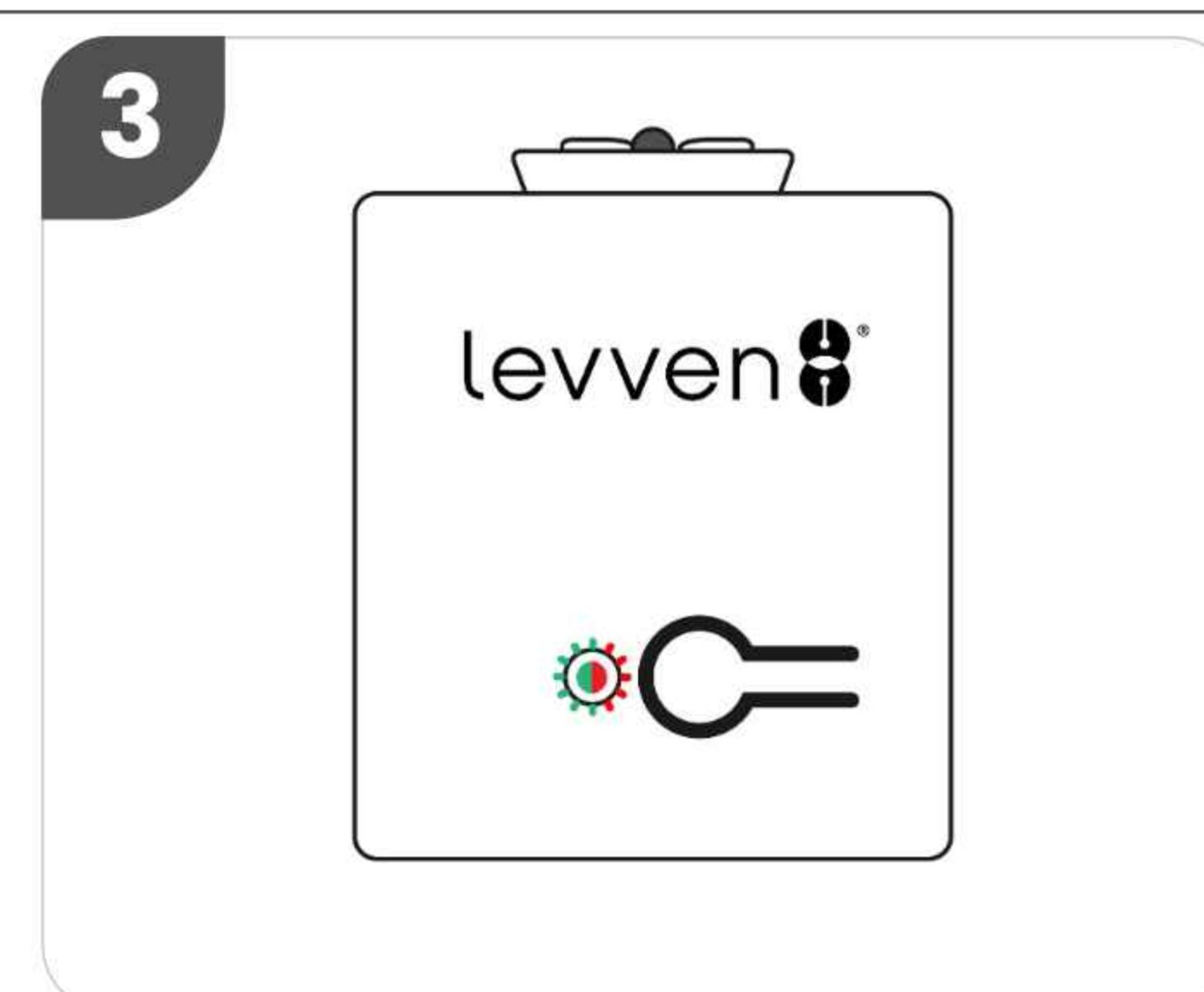
The LED on the controller will start blinking red and green to confirm a signal is received.
