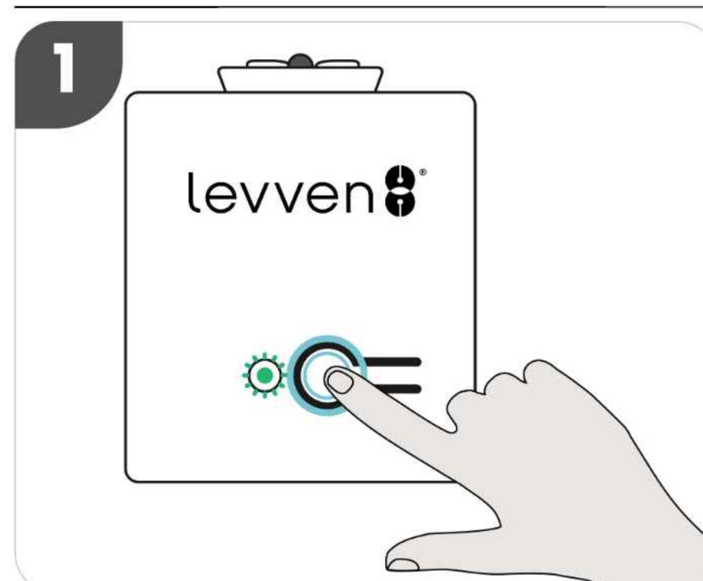
Press and release the pair button on the controller to initiate pairing. This controller's LED will blink green. The pairing mode is active for 60 seconds. If no pairing request is received within 60 secs, the controller exits pairing mode.
