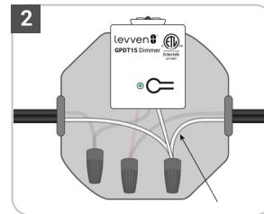
Connect the white wires from the power, load, and power controller together.
