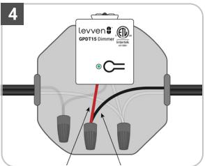
Connect the black load wire to the red wire of the power controller.
