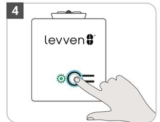
Press and release the pair button on the controller to complete pairing. Its LED will flash green 3 times to confirm pairing.
